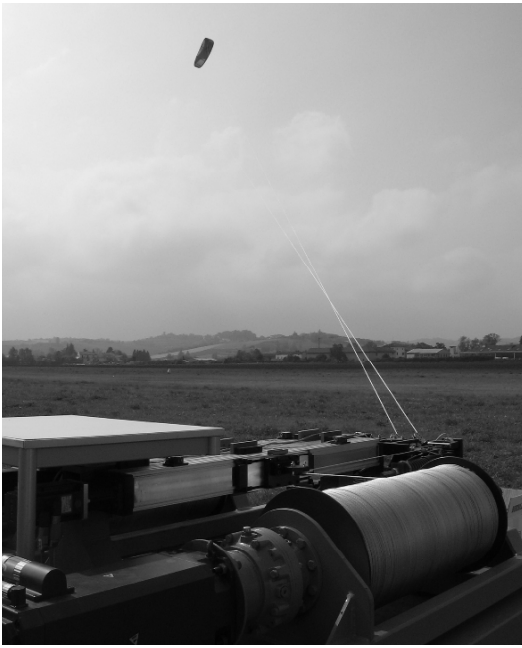
Fig. 4. KE-yoyo small scale prototype operating near Torino, Italy.
