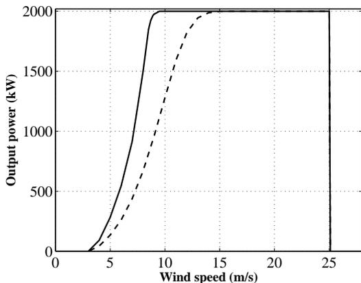
Figure 3: Comparison between the power curves of a typical wind tower (dashed) and of a KE-yoyo (solid), both with the same rated power of 2 MW.
