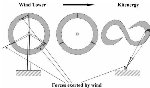
Figure 1: Basic concept of Kitenergy technology
