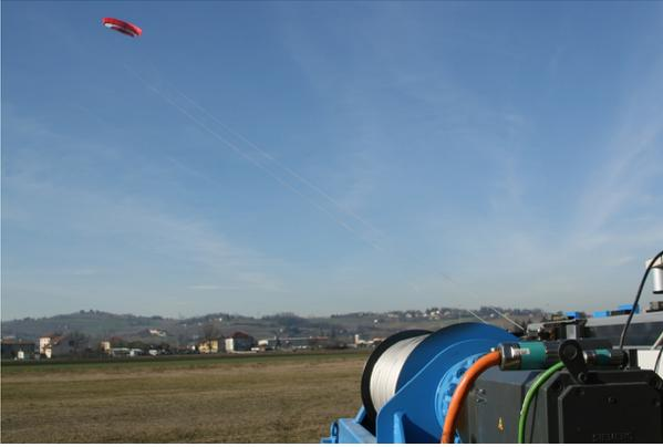
Figure 4: KE-yoyo small scale prototype operating near Torino, Italy.
