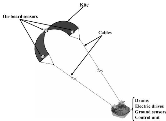
Figure 2: Scheme of a Kite Steering Unit (KSU)
